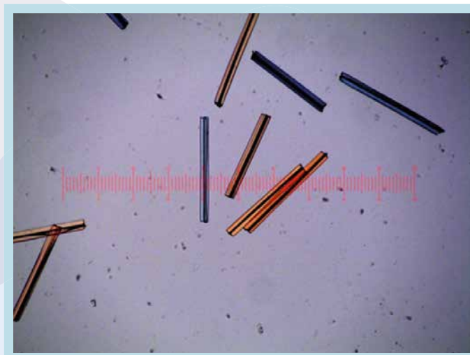
Figure 2. Light microscopy photomicrograph of rayon fibres, 500 x 44 \mu\text{m} (fibres were kindly supplied by Minifibres Inc, Florida, US).
